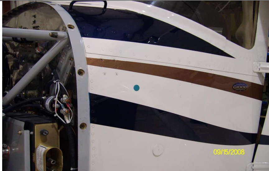
Blue dot is Typical (Optional) Piezo Electric Switch Installation
