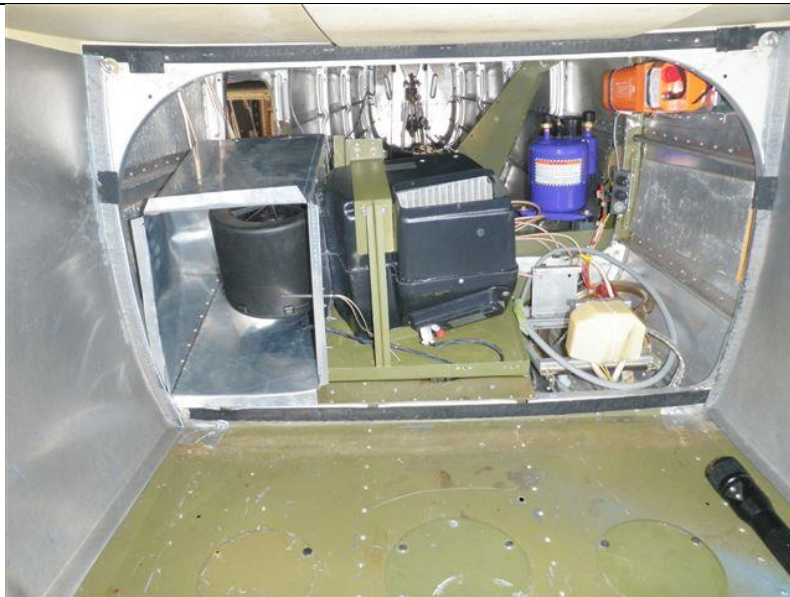
Figure 8 - Evaporator Assembly Installation 182Q
