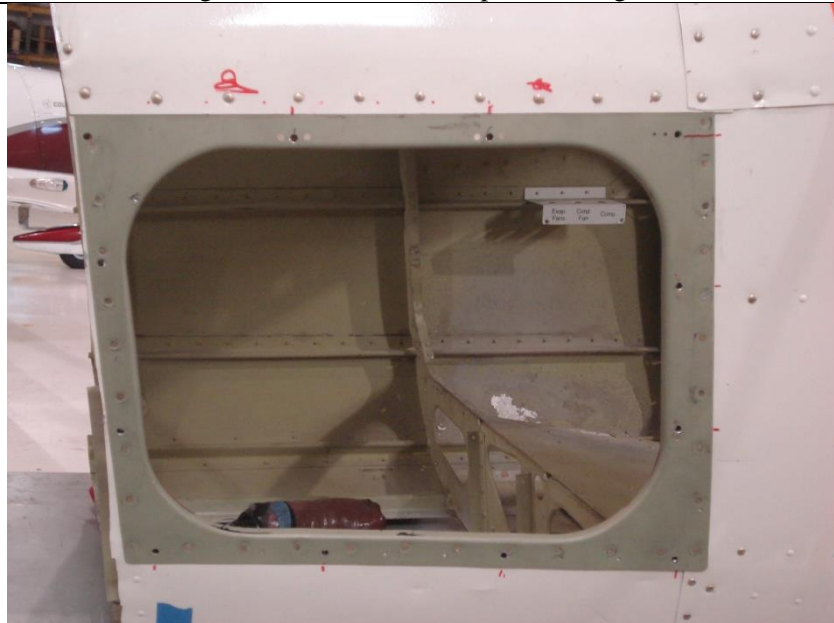
Figure 4 - Install Access Panel Doubler
