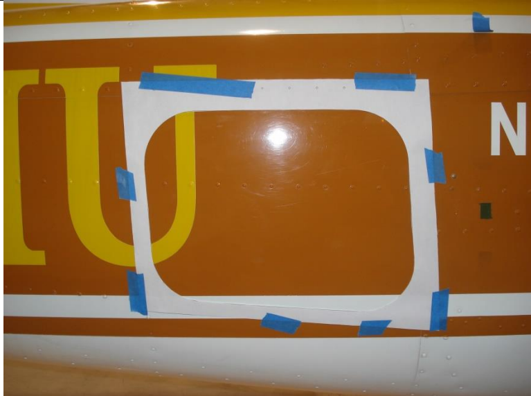
Figure 1 - Access Panel Template
