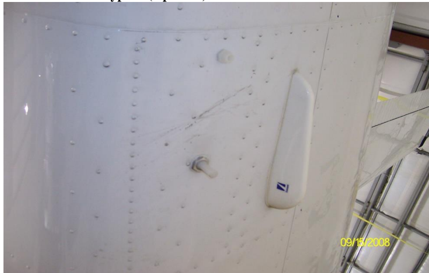
Aft Most Drain (top of picture) Line is Typical Evaporator Drain Installation
