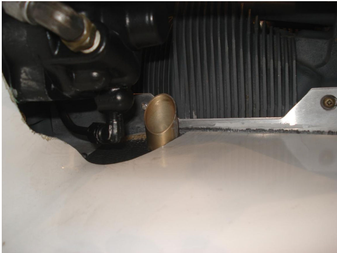
Figure 9 - Cowl modification for blast tube.
