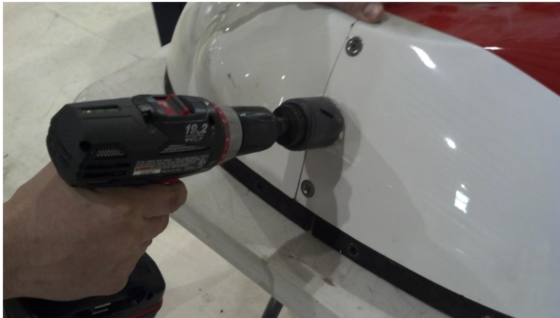
Figure 5 - Cowling Clearance Hole Location
