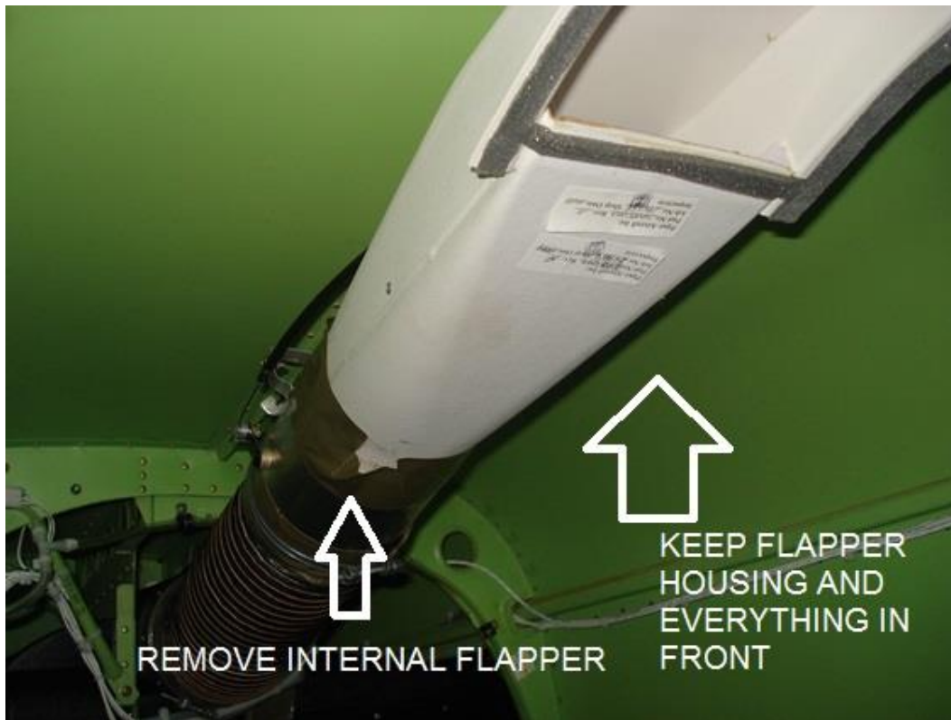
Figure 2 – Existing Fresh Air Vent Removal
