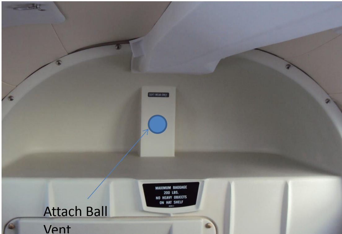
Figure 7 - Ball Vent Location
