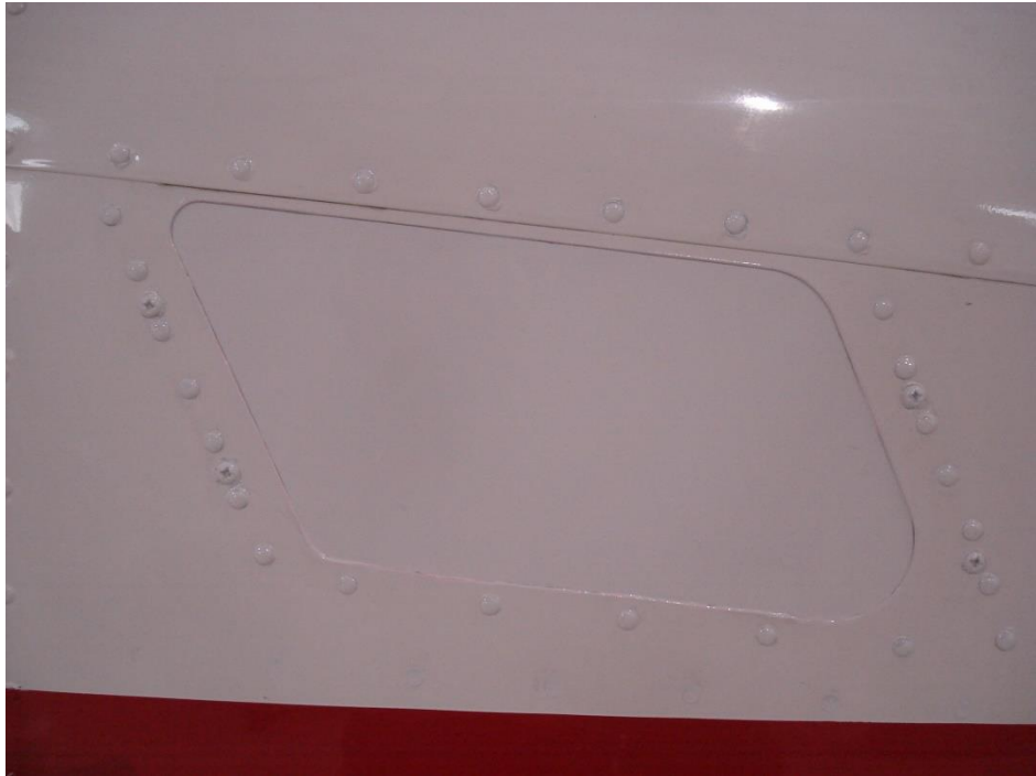
Figure 3 – Air Inlet Cover Installation
