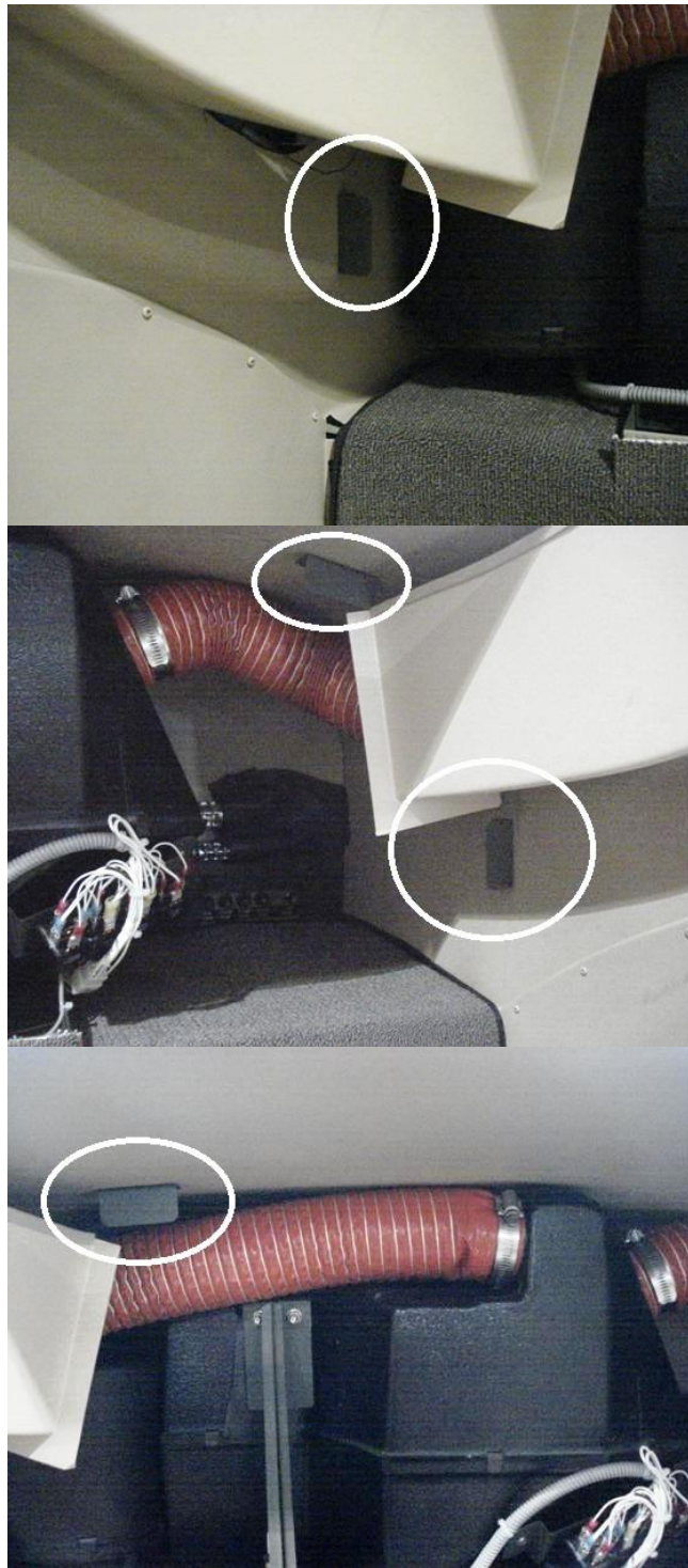
Figure 15 - Evaporator Blockoff Brackets
