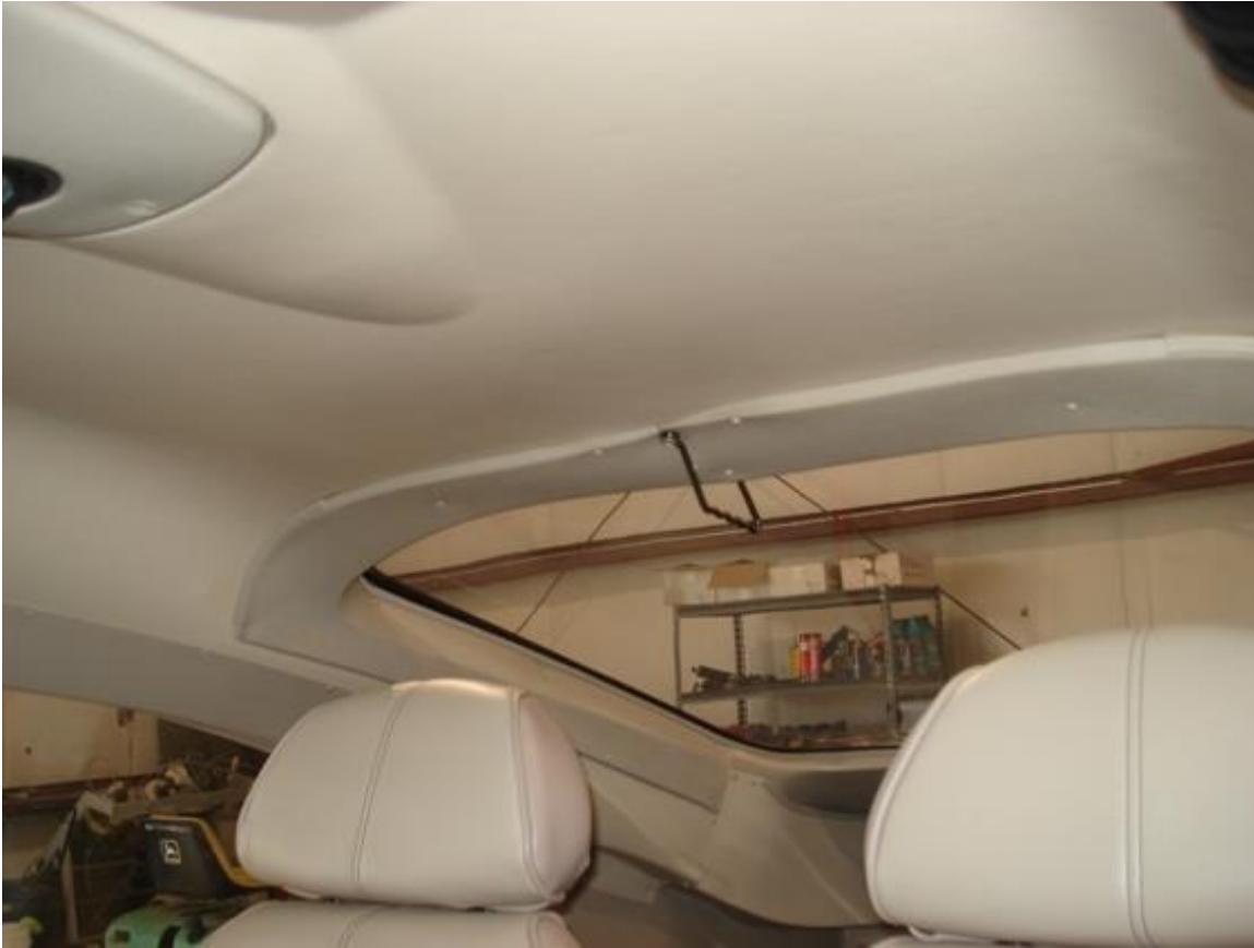
Figure 14 - Rear Window Trimming
