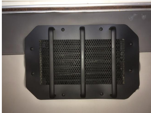
Figure 19 – Cabin Inlet Doubler Installed
