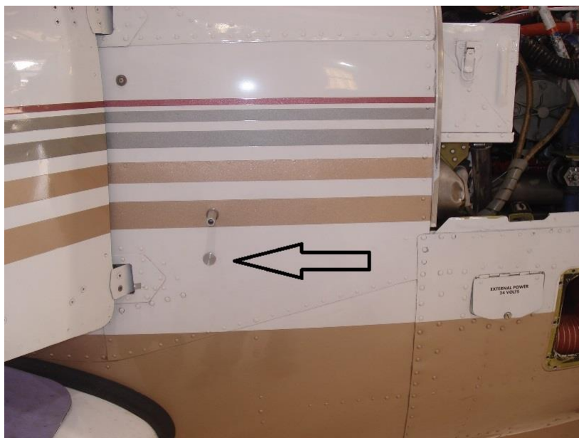
Figure 24 – Bonanza Piezo Switch Installation
