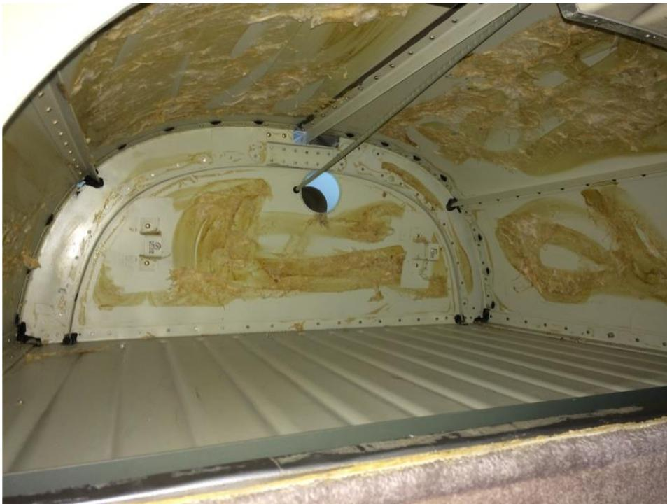
**Figure 27 - Air Duct Removal**
