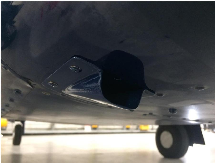
**Figure 33 - Attached Drain Scupper**
