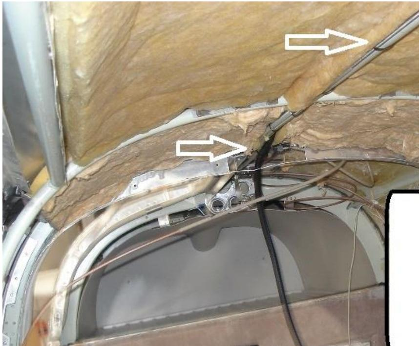
**Figure 24 – Climate Control Extension Harness Routing**
