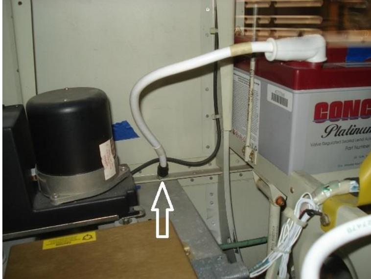
**Figure 40 – Wire Routing**
