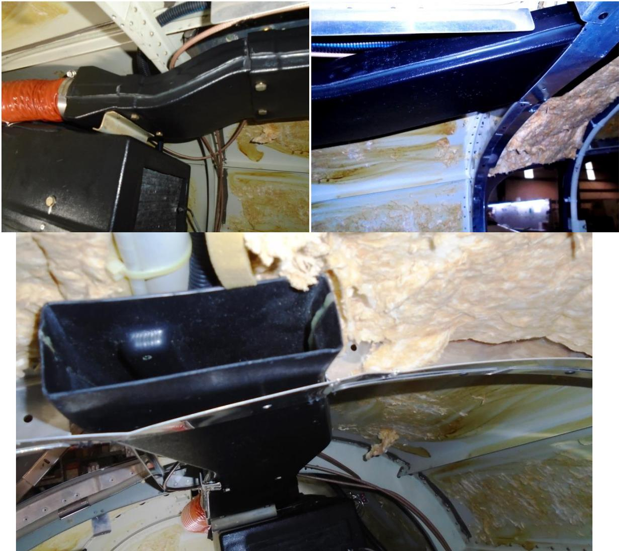
**Figure 35 – Outlet Upper Duct Installation**
