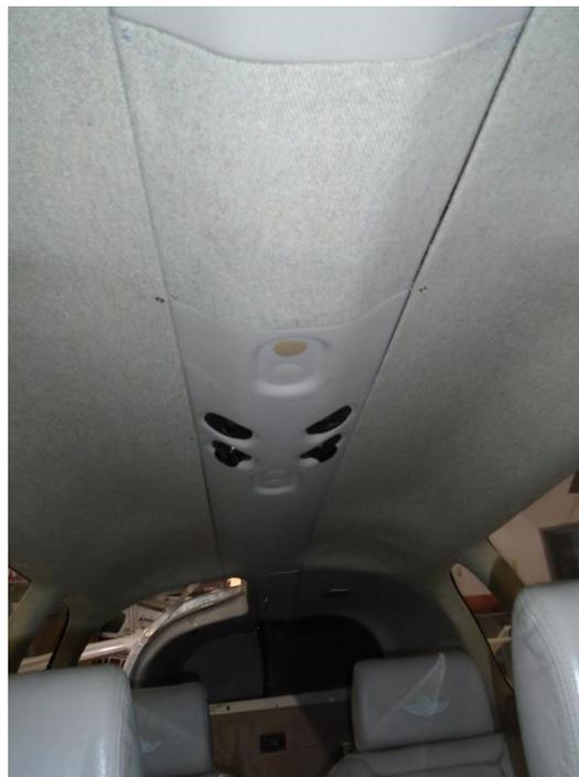
**Figure 37 – Headliner Reinstallation**
