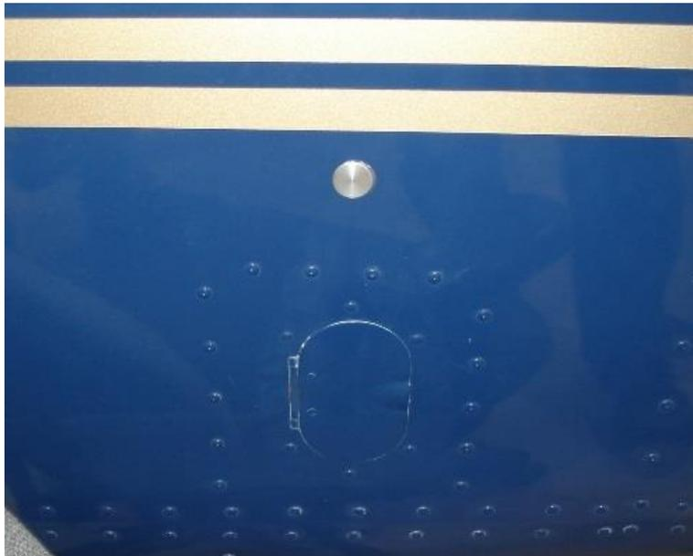
**Figure 43 – Mooney Piezo Switch Installation Exterior View**
