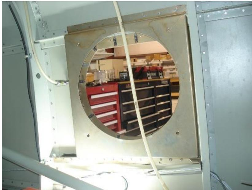
**Figure 6 – LH Sidewall Condenser Hanger
