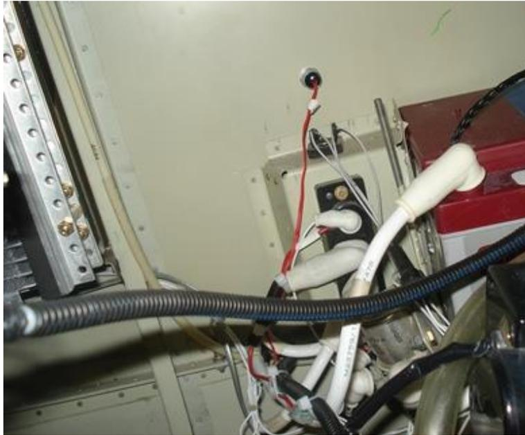
**Figure 42 – Mooney Piezo Switch Installation Interior View**
