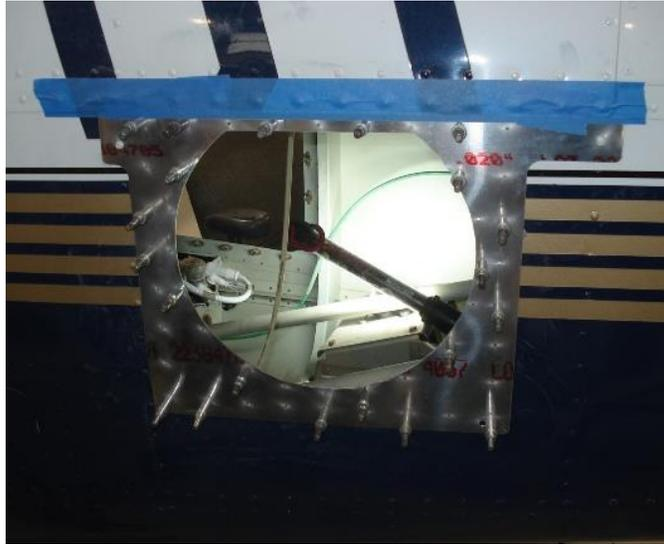
**Figure 1 – LH Sidewall Cutout Template**
