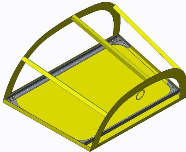
**Figure 29 - Evaporator Support Structure**
