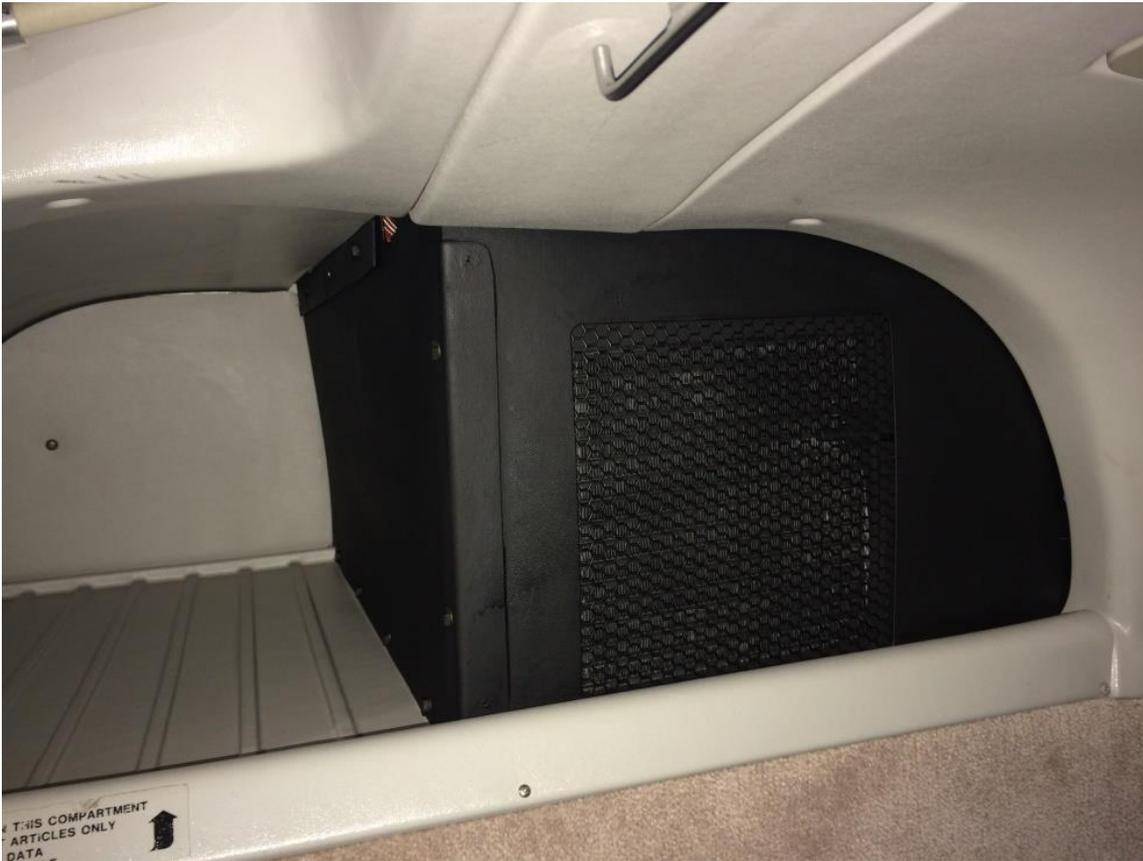
**Figure 38 - Completed Evaporator Installation**
