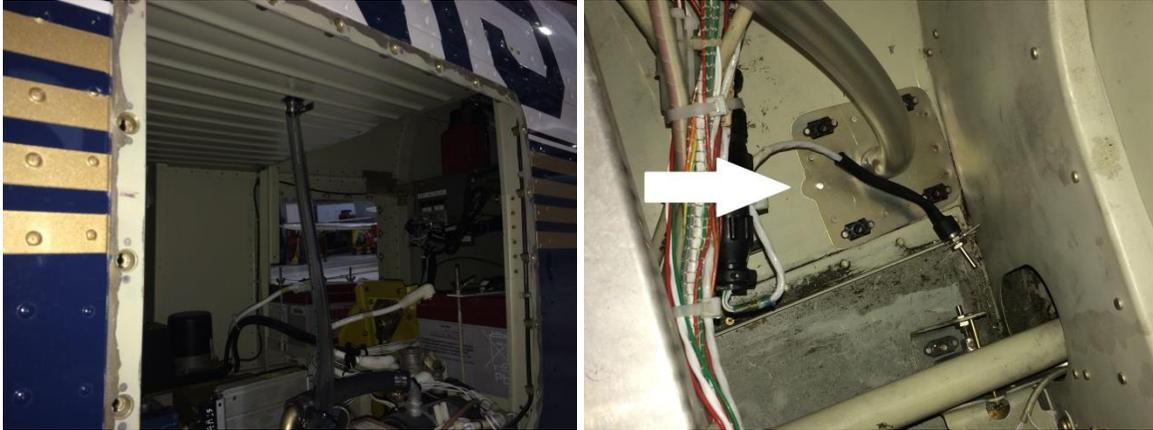
**Figure 32 – Evaporator Drain**
