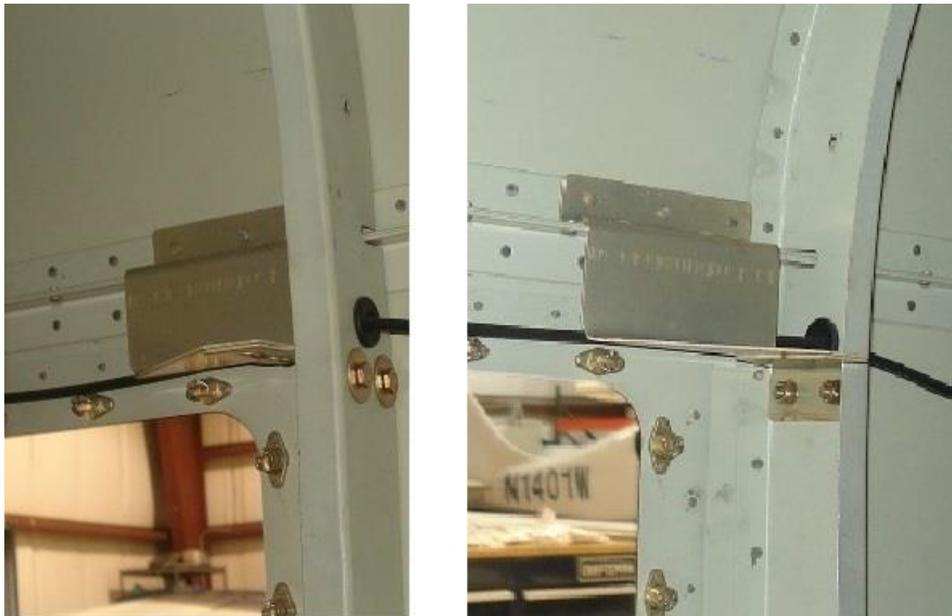
**Figure 4 – Compressor Support Bracket Installation**
