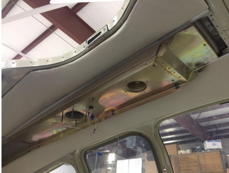
Figure 6 - Install Forward Duct Assembly
