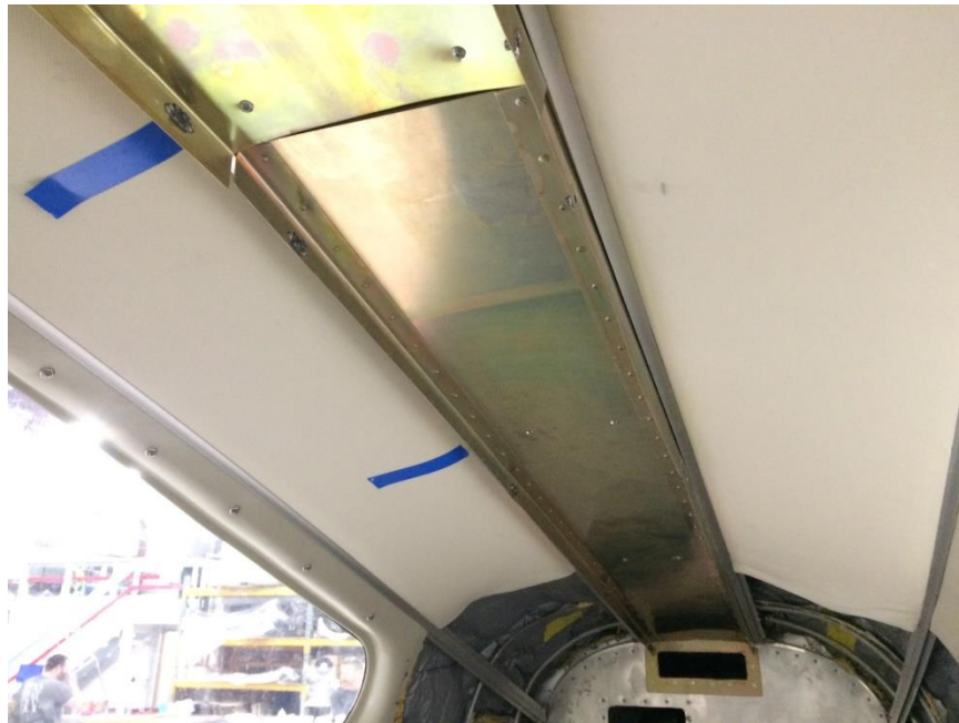
Figure 5 – Install Rear Duct Assembly
