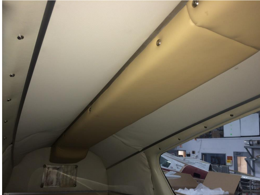
Figure 8 – Install Rear Duct Cover
