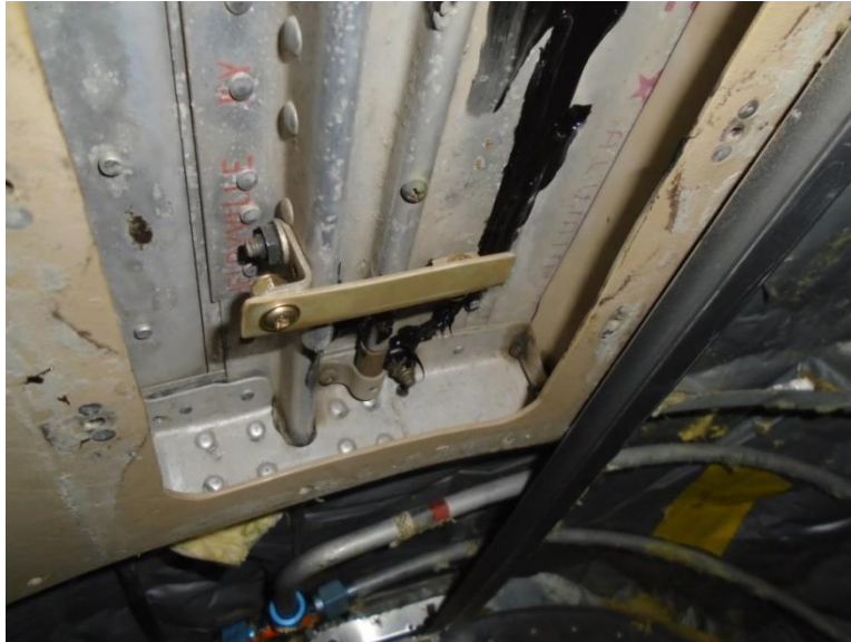
Figure 1 - Seal Vent Door Closed
