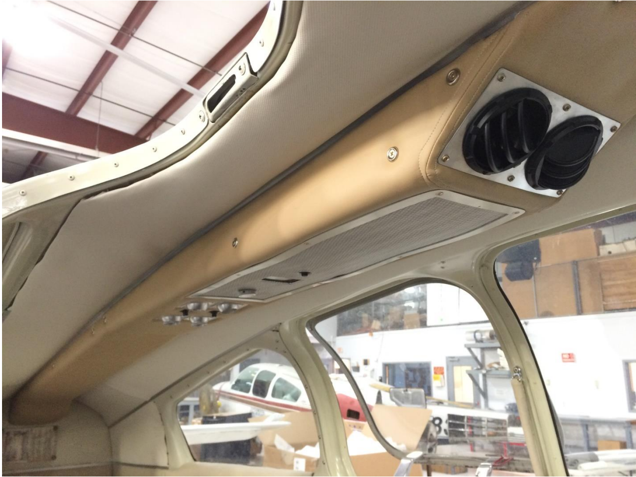
Figure 12 - Completed Headliner Installation
