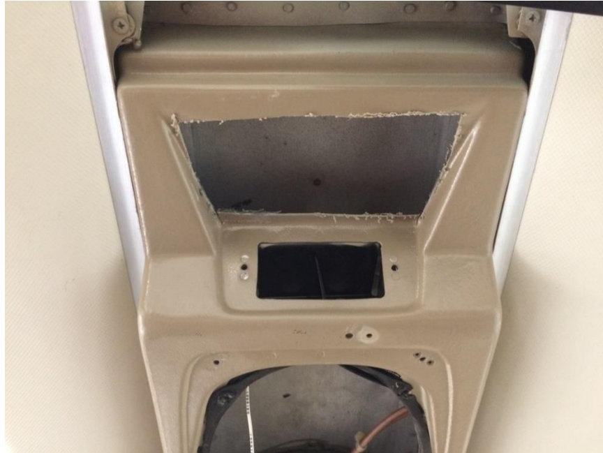
Figure 4 - Remove Map Light and Vents
