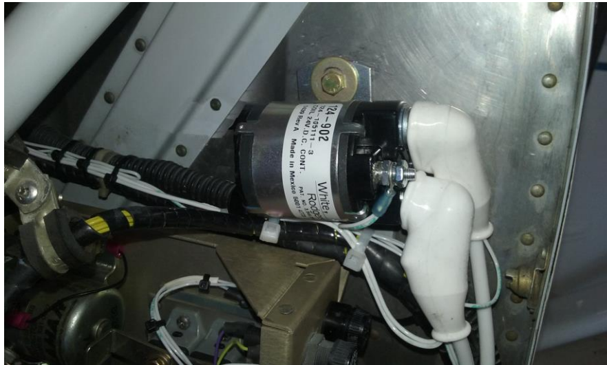
Figure 2 - Mounting location of DC Contactor Relay
