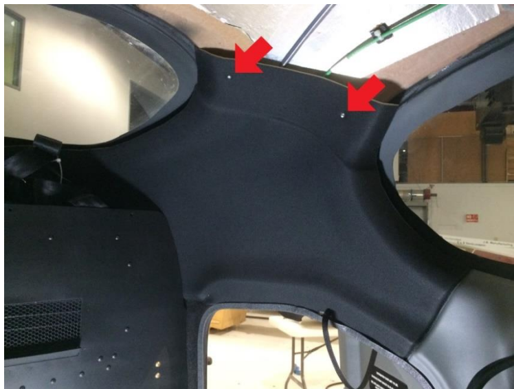
Figure 4 - Left Rear Panel installation
