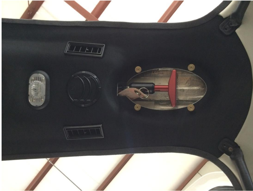
Figure 7 - Headliner, pillar and trim installation
