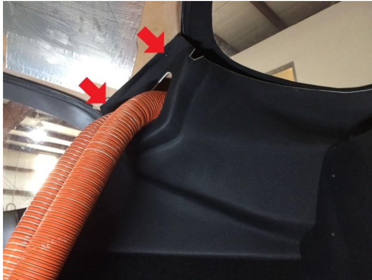
Figure 3 - Attach tubing, feed through Right Rear Panel then fasten
