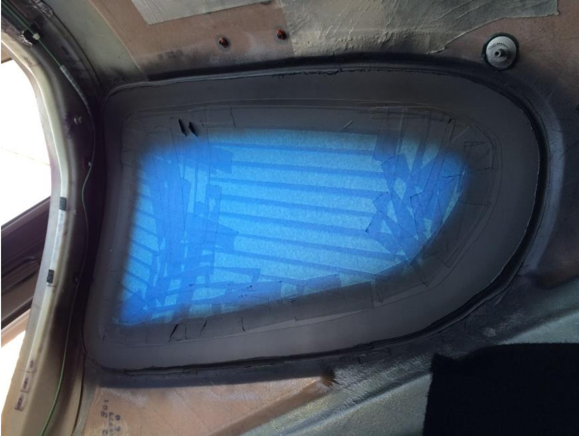
Figure 2 - Mask windows and paint border if required
