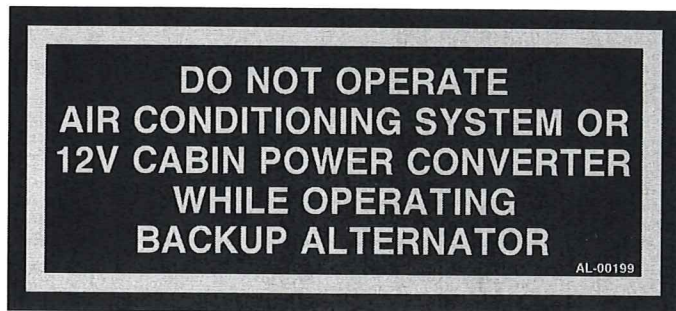
Figure 1 - Backup Alternator Limitation Placard
