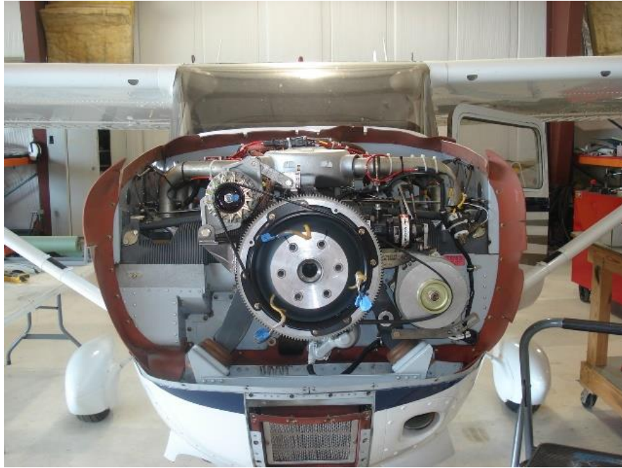
Figure 4 – Alternator Installation and Belt Placement
