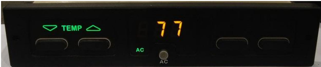
Figure 2 – A1235 Controller Front Panel – AC Mode
