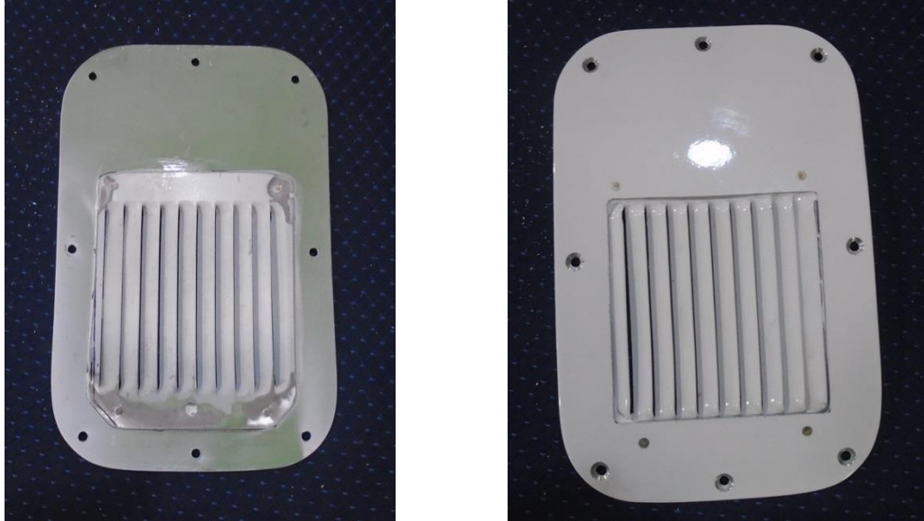
Figure 16 – F3 Tail Cone Vent Modification
