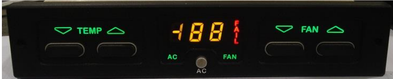
Figure 3 – A1235 Controller Front Panel - Self Check Mode
