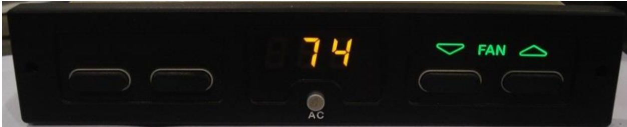
Figure 5 – A1235 Controller Front Panel – Fan Mode
