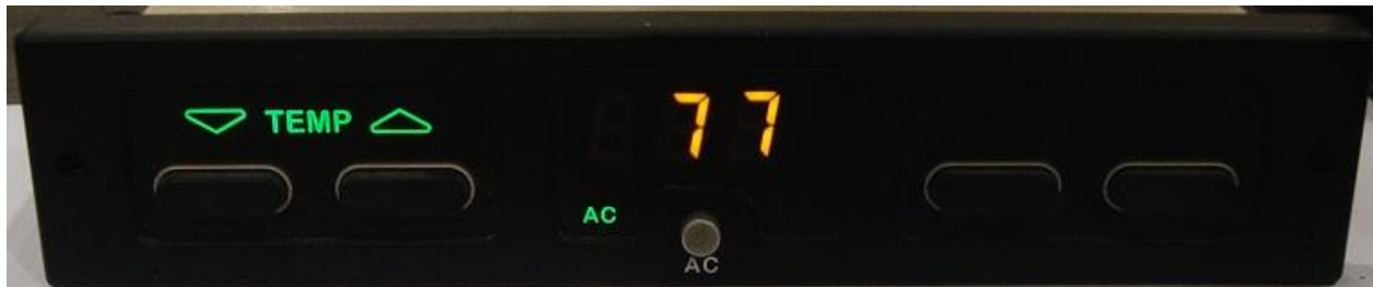
Figure 4 – A1235 Controller Front Panel – AC Mode
